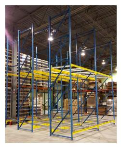
A Roll Form Push Back Pallet Rack Systems may feature skate wheels that divide the beams into product lanes. When a pallet is loaded onto the beam, it pushes an existing pallet back. When a pallet is removed, the pallet(s) behind it roll forward.
